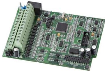
Inverter Control Board
